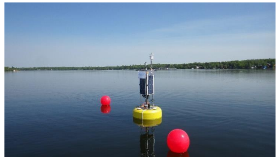
Example of a lake monitoring buoy installed on Nakamun Lake in 2019.
